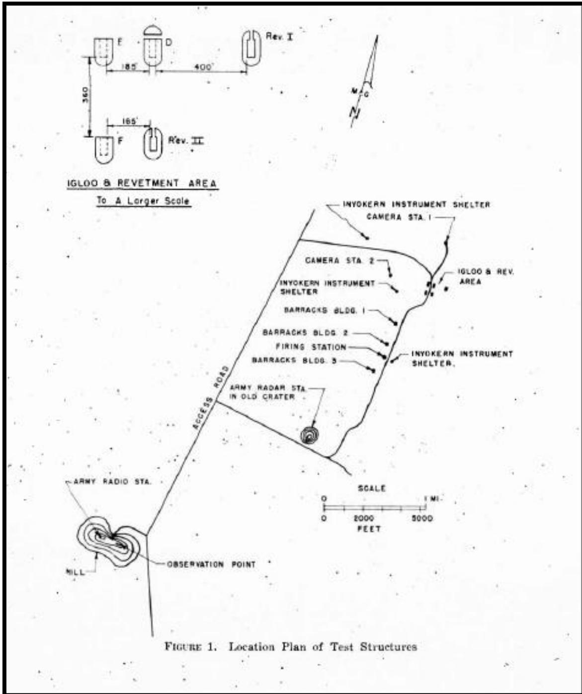
FIGURE 1. Location Plan of Test Structures
