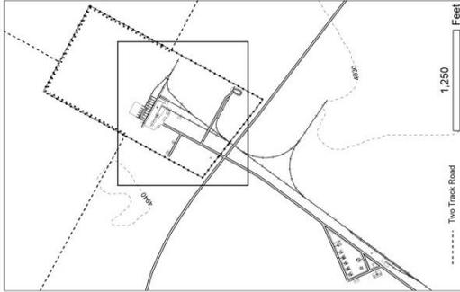
In 1943 the proofing area at the Arco NPG provided for 10 gun emplacements of various types. The railroad spur from Scoville junction brought guns directly to the emplacements where they were stored in concrete structures. The structures were located at the southeast end of the emplacements. A transfer track could then move guns to the appropriate emplacement for testing.
