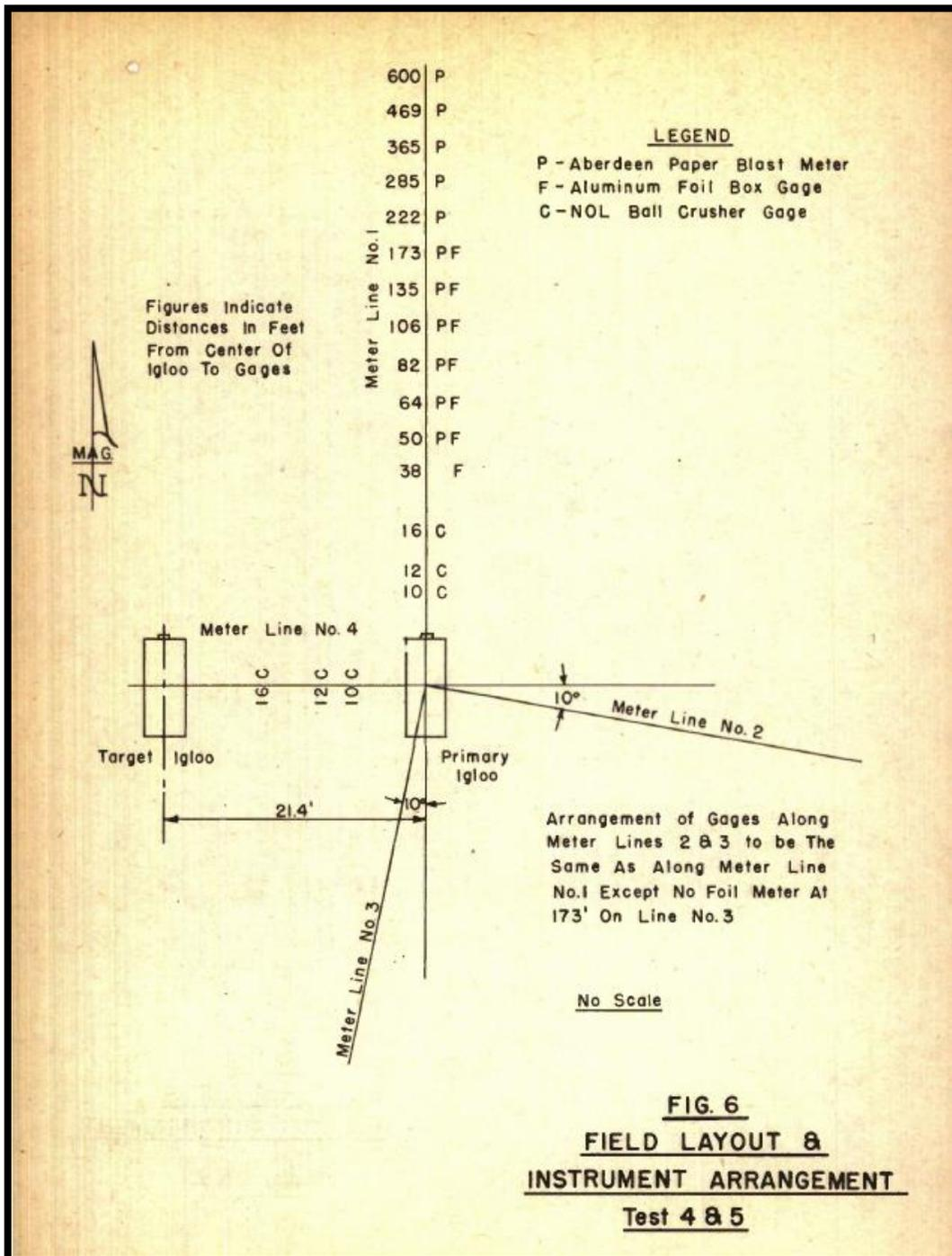
Figure 5.189: "Field layout and instrument arrangement tests 4 and 5", ANESB scale model igloo tests, 1946 (Mann 1947, 8).
